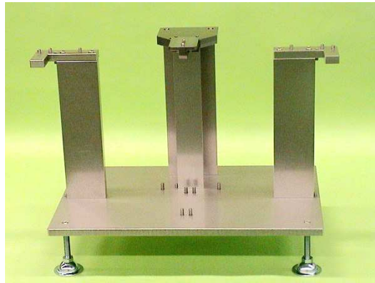
Drw. S1.2-1 Joint initial setting jig
