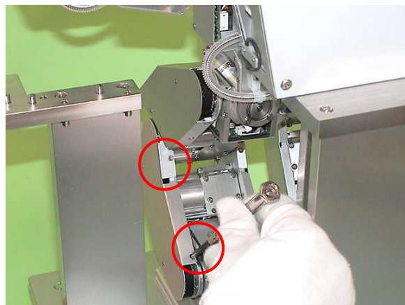
Drw. S1.5-3 Fix position of the outside leg cover
