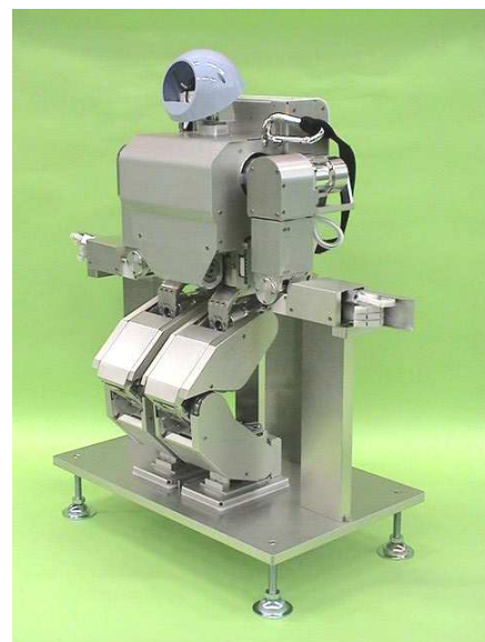
Drw.1.2-2 Initial posture of robot to be standard when fixed on joint initial setting jig.
