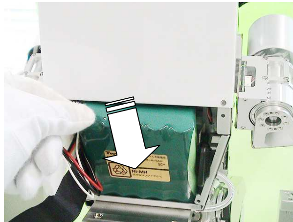
Drw. S1.4-4 Install the battery
