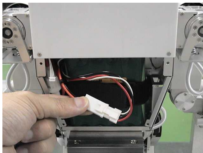
Drw. S1.3-2 Removed the back cover
