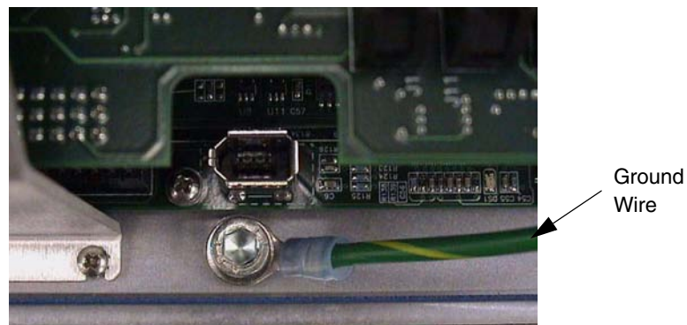
Figure 8-4. Ground Screw on AIB Chassis
