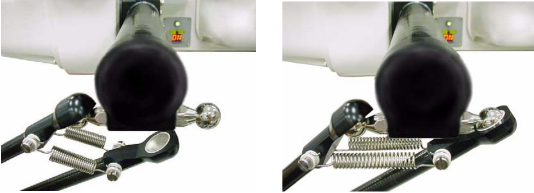
Figure 3-9. Installing Ball Joints
