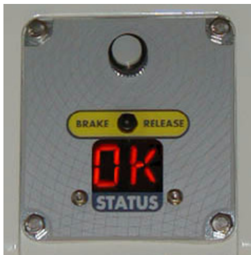
Figure 8-5. Status Display Panel, Showing 4 hex-head Screws
