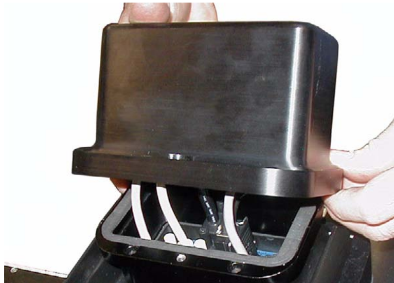
Figure 9-12. Installing Cable Entry Top Cover Assembly
