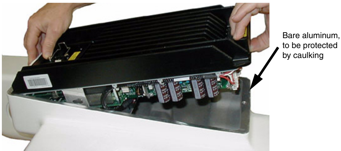
Figure 9-1. AIB and Base, Showing Non-anodized Aluminum
