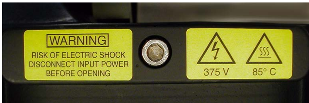
Figure 2-1. Electrical and Thermal Warning Labels on AIB Chassis
